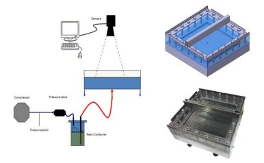
Fig. 3: Permeability test bench set-up (left), injection mould (right)
