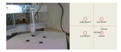
Fig. 2: Anode-to-cathode-system (left), welding spot location and contact pressure (right)
